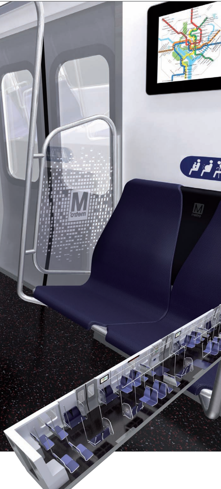
LEFT: The 7000 series eschews central poles, seatback grab handles and headrests for an open feel
