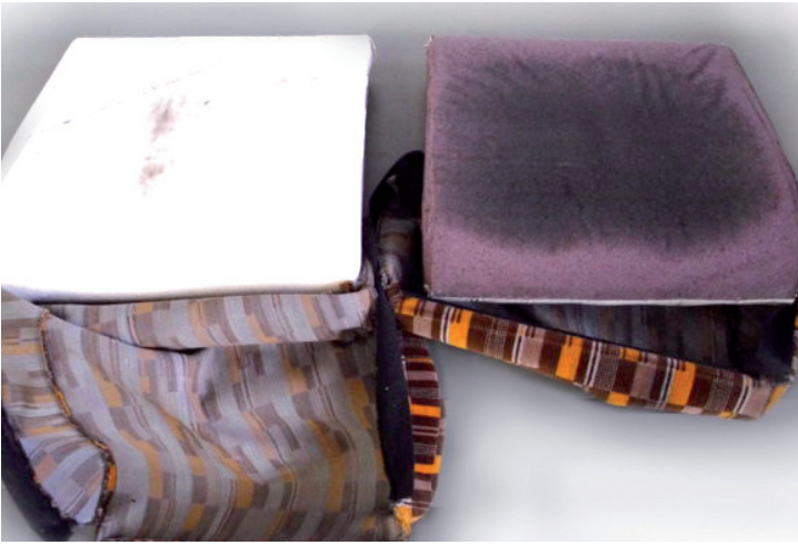
ABOVE: After a 100,000-cycle test, the silicon foam (on the left) remains largely unchanged
