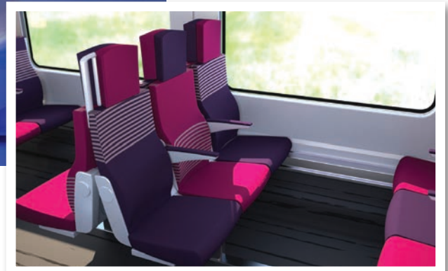
ABOVE: The Francilien’s seats are cantilever-mounted so bags can be put underneath
