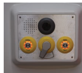
ABOVE: The fittings are designed for use by visually impaired and elderly passengers
