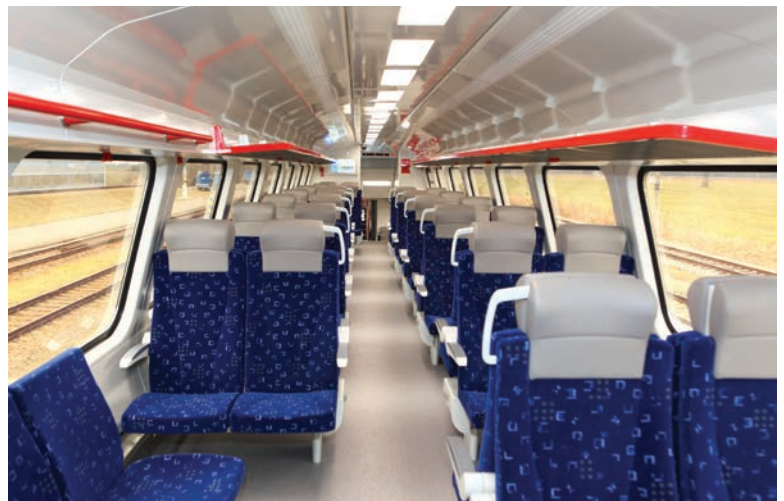
TOP AND ABOVE: Regio seats installed on a double-deck train
