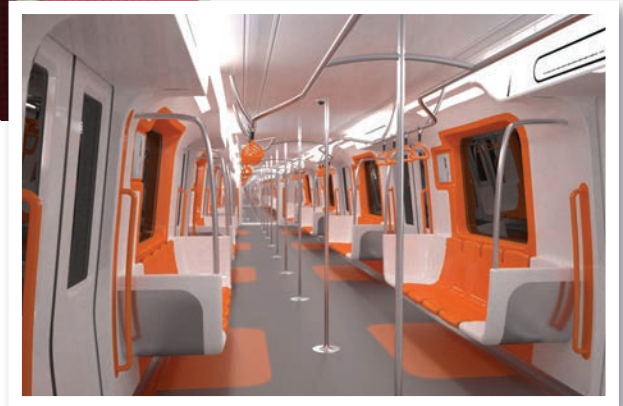
RIGHT: MBD’s design for a Chinese train features lots of handrails for standing passengers
