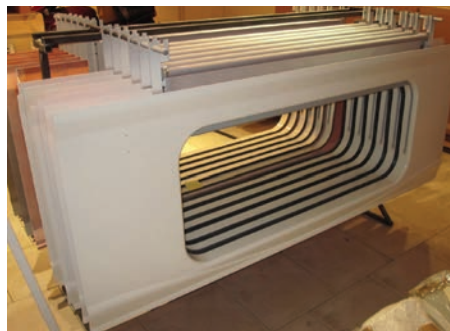
ABOVE: Phenolic window panels for Alstom's Pendolino
