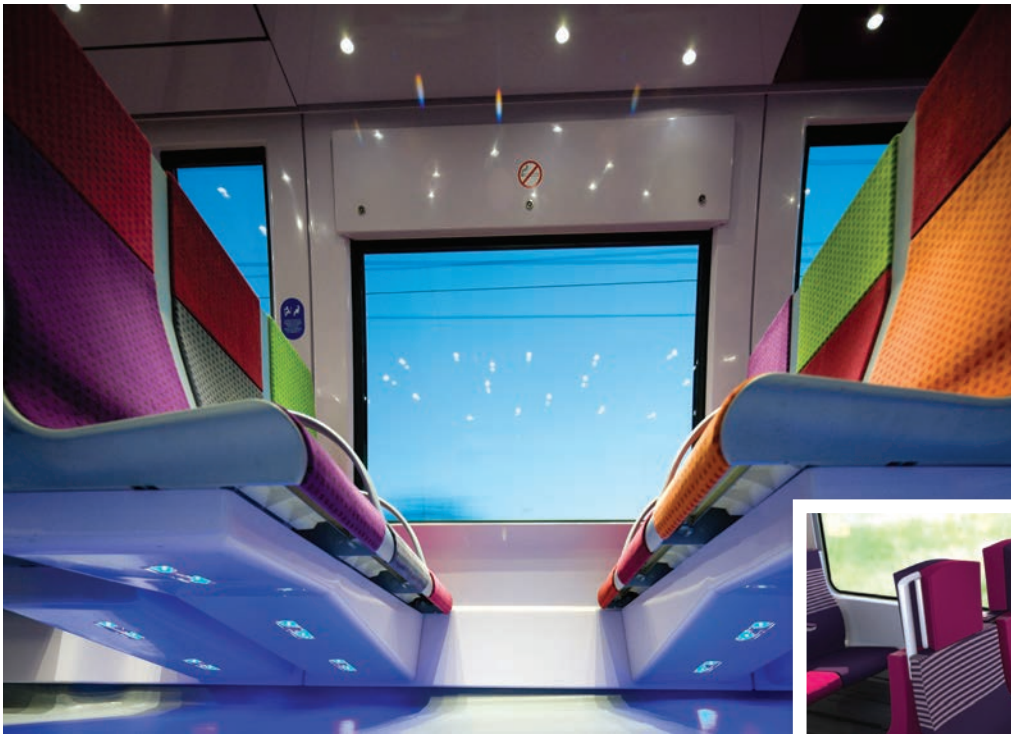
ABOVE: The Francilien’s seats are cantilever-mounted so bags can be put underneath
