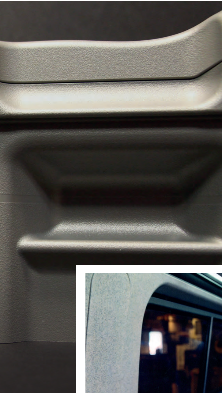
ABOVE: Vacuum-formed (left) and pressure- formed (right) thermoplastic
