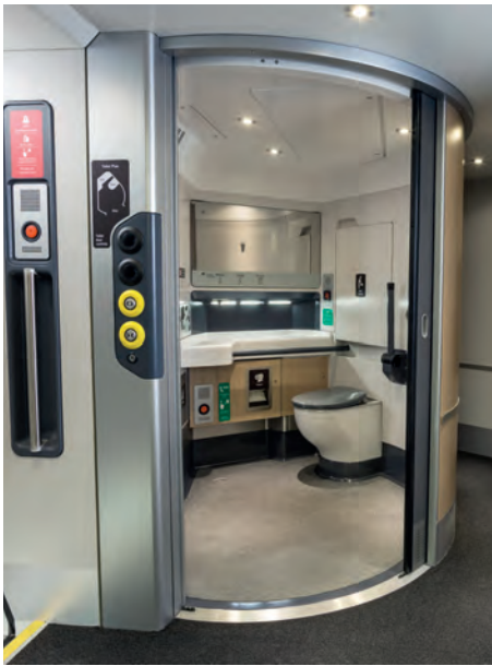
ABOVE AND RIGHT: A universal access toilet designed by DCA and Hitachi for the UK's IEP
