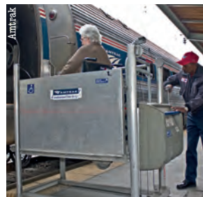
BELOW: For boarding, Amtrak can provide a ramp or, as shown, a mobile lift
