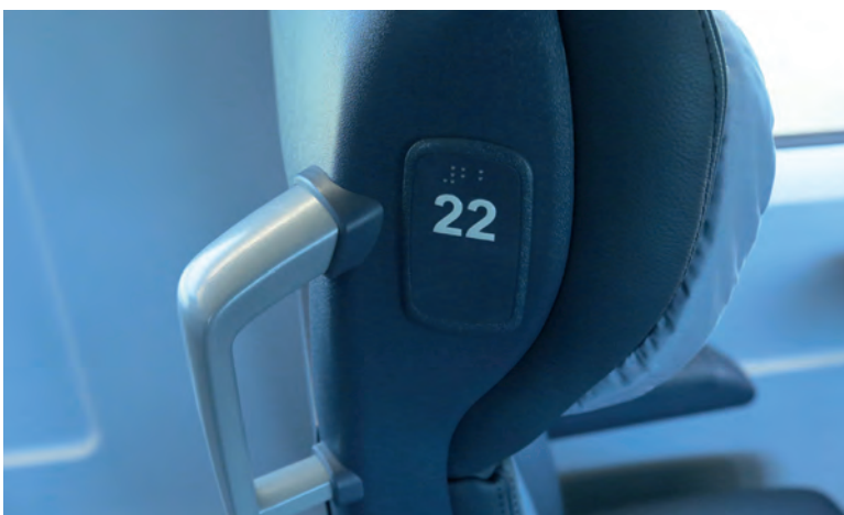
LEFT AND CENTER: Signs, seat numbers and car numbers are provided in braille on Siemen's new Velaro D/ ICE train for Deutsche Bahn
