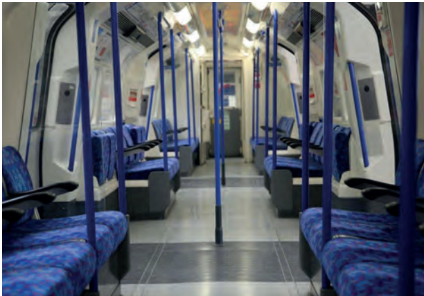
LEFT: Two colors of TM7 were co-vulcanized for a seam-free finish on London Underground's Northern line
