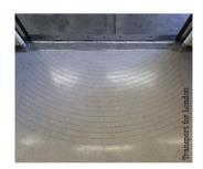
ondon Underground transports approximately 1.3 billion passengers every year and so a heavy-duty floor covering is essential – and it also fulfills a critical safety role. The most recent project undertaken by Treadmaster for London Underground involves the supply of more than 9,000m<sup>2</sup> of its TM7 flooring product for the refurbishment of 36 seven-car metro trains (built in 1972) on the Bakerloo line.
