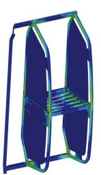
RIGHT: A simulation conducted by Siemens to test a baggage rack
