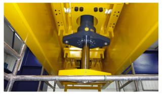
LEFT AND ABOVE LEFT: Equipment at the Centre for Innovation in Rail includes these vertical actuators, used to simulate vehicle body dynamics for the bogie under test
