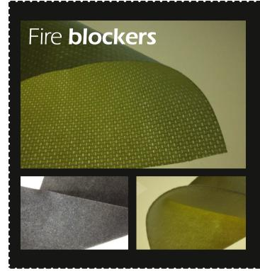
he custom-engineered spun-laced and needle-punched materials offered by Norafin are suitable for use as fire blockers in a range of markets, including public transport. Norafin says these technical non-woven materials' fire blocking and fire retarding capabilities accord with EN 45545-2, FAR/CS25.853a, ABD 0031-F and BSS 7239 standards, and the materials also comply with railway standards regarding the emission of smoke and toxic gases.
