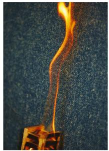
of testing and their own requirements for fabrics. The UK, for example, has to meet the BS 6853: 1999 standard, a code of practice for fire precautions in the design and construction of passenger-carrying trains. The standard provides varying criteria for every component used in a rail carriage.
