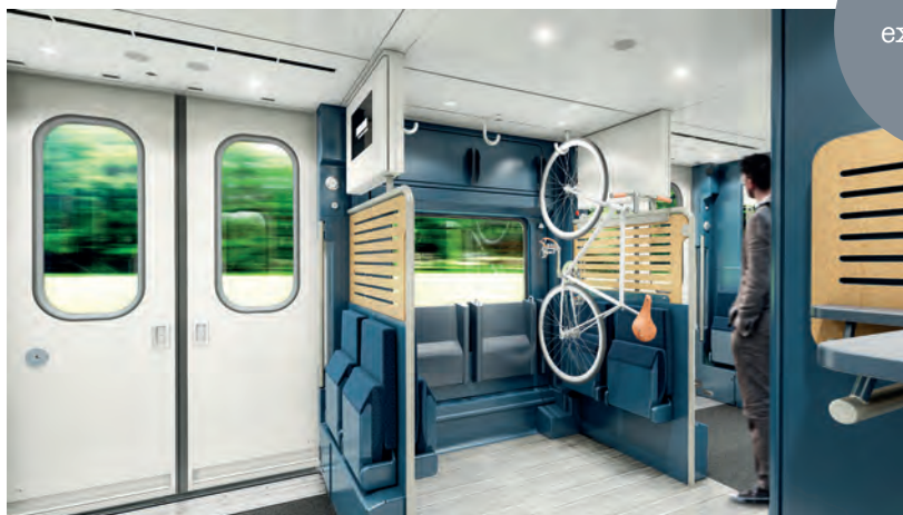
ABOVE: The PRM area LEFT: The bike racks integrate tip-up seats, helpful for those using the refreshment area opposite
