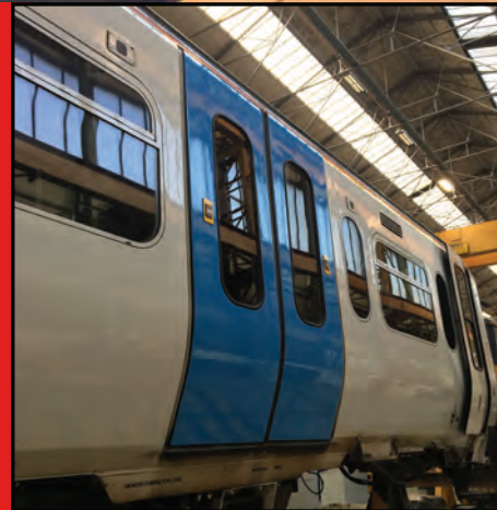
Doors with No Delamination or Corrosion
