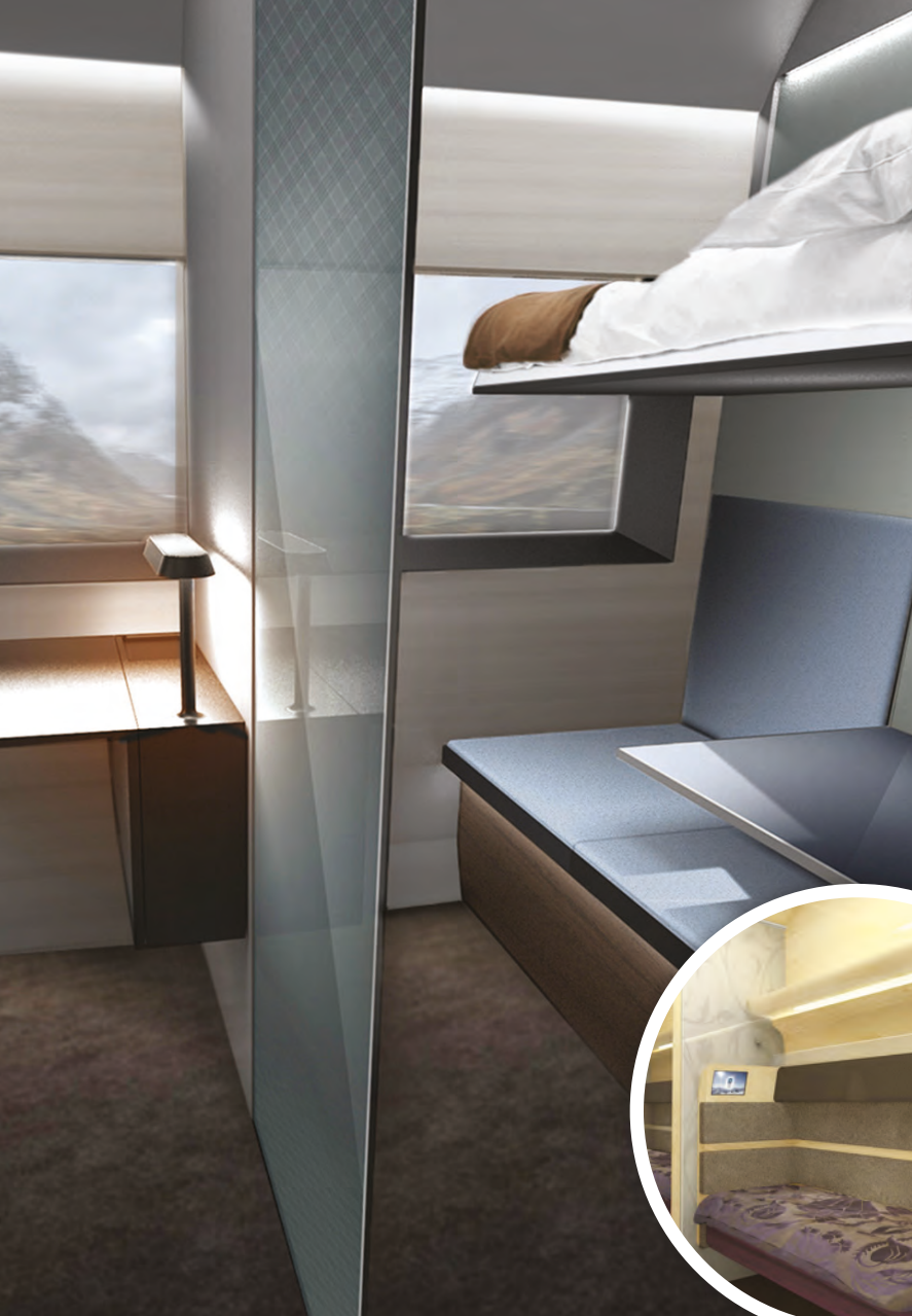
LEFT: A concept by tangerine for an adaptable berth with a moveable partition, enabling flexible arrangements for families
